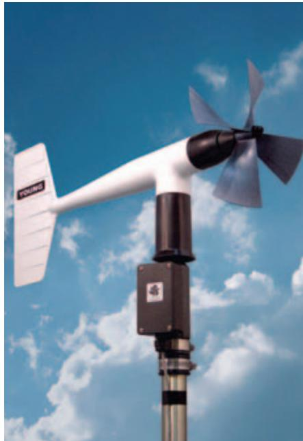
Wind speed is sensed by a lightweight, carbon fiber thermoplastic (CFT), helicoid propeller. Propeller rotation produces an AC sine wave voltage signal with frequency directly proportional to wind speed. Slip rings and brushes are not used.
